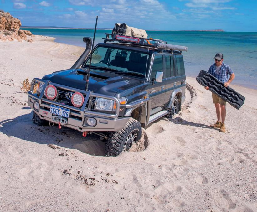
Designed, developed and manufactured in Australia, TRED Pro recovery boards are the result of years of consumer feedback and in-the-field testing. They are made from a dual-composite material that provides flexibility across the board as well as incredible strength on the grip nodules that could otherwise be damaged by wheel spin.
