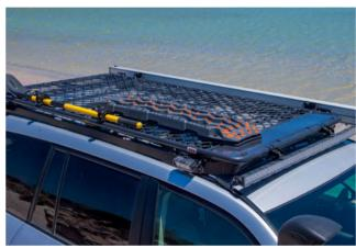
The shape of TRED Pro changes from concave to convex along its length, which is designed so the tyre can more easily pull the vehicle out of its predicament once momentum has been built up.
