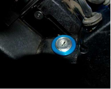
Screw the Blue Aluminium Bezel over the thread on the column sleeve. A little grease on the threads makes this much easier as the threads are deliberately tight. If you find you cannot grip the bezel tightly enough, wrap some tape, sticky sire out round your finger tips. this will help you grip the bezel without damaging it.
